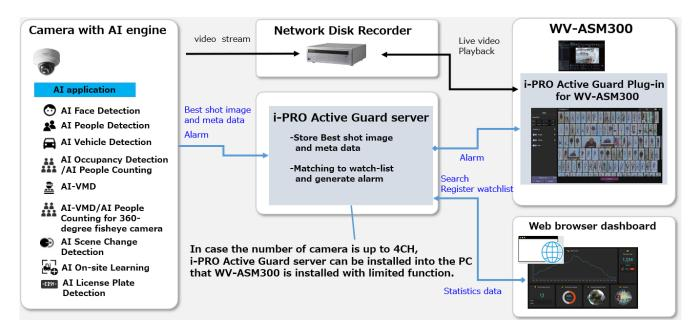
Al application or Al function on cameras transmit video stream to VMS server/Recorder and transmit Best shot images and meta data to i-PRO Active Guard server.
