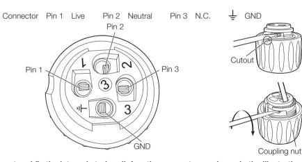
(5) Insert and fix the internal strain relief on the connector as shown in the illustration. Next, rotate the screw of the internal strain relief, and fix the power cord firmly with the fixing bracket.
