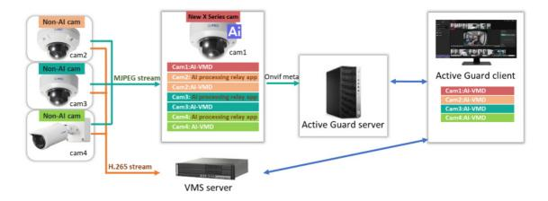
This product is software for more convenient use of AI network cameras (sold separately). By installing this product on a camera, configuring non-AI camera settings, and configuring the extension software, AI processing can be performed on video from cameras that do not have AI functions.
