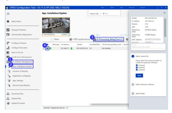
The following procedure is the operation of the "AI Processing Relay(Cam.2-)" screen. There is no installation order for Camera 2, Camera 3, and Camera 4 extension software.
