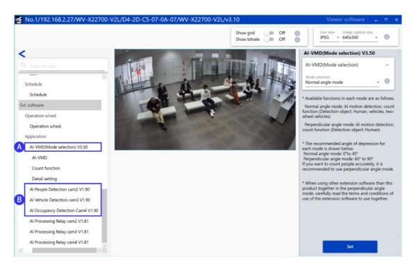
The images of non-AI cameras (Camera2, Camera3, and Camera4) are not displayed on the configuration screen of the software for Camera2, 3, and 4. If you need to make settings while viewing the images, click the link (C in the figure below) displayed on the iCT screen and make settings on the browser's settings screen.
