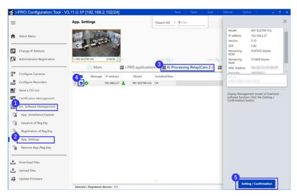
2. The detailed settings screen of the Extension Software will be displayed. Scroll through the menu on the left to the "AI Processing Relay CamX Vx.xx" item.
