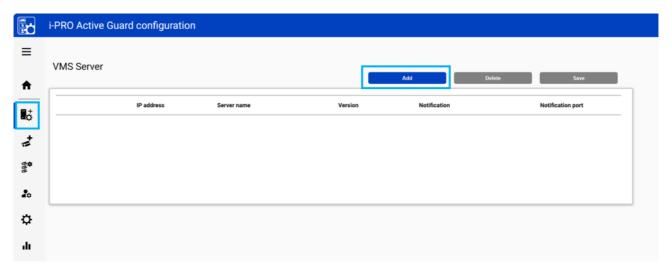
2. Press the "Test" button after entering the VMS information. When "Success" is displayed, press the "Save" button.
