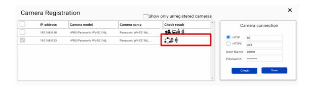
When the 3<sup>rd</sup> party extension software is installed in the selected camera, icon will be shown in the [Check result]. If not shown, please check if configuration file is edited correctly.
