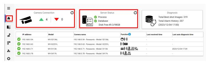
means the number of cameras connected. (Meta data session between camera and i-PRO Active Guard server).
