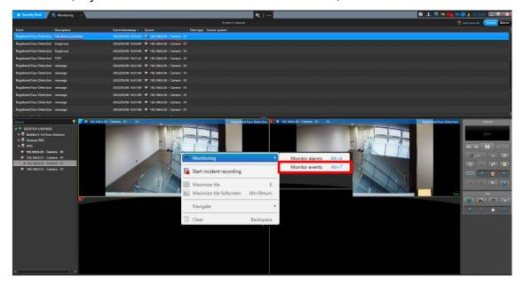
"Registered face detection", "Registered people detection", "system alarm of i-PRO Active Guard server", and etc event can also be shown as "Alarm" by configuring [Alarm] and [Actions].
