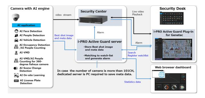
Al application or Al function on cameras transmit video stream to Security Center and transmit Best shot images and meta data to i-PRO Active Guard server.
