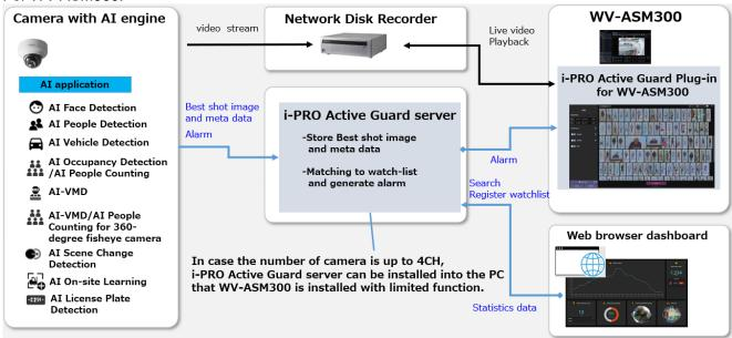
Al application or Al function on cameras transmit video stream to VMS server/Recorder and transmit Best
