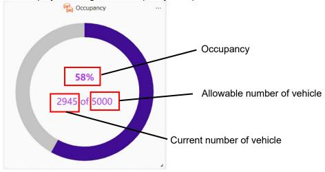
**Occupancy:** Shows how crowded the aggregation target area is. Current number of vehicle ÷ Allowable number of vehicle (%).
