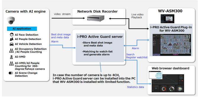
Al application or Al function on cameras transmit video stream to VMS server/Recorder and transmit Best
