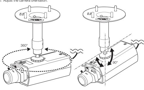
3 Turn the hexagonal hole with a hexagonal wrench to tighten the fixation of the movable part. Hexagonal wrench (3 mm on each side) (procured
