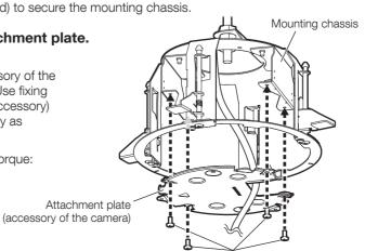
Fixing screw for attachment plate (4 pcs.) (M4: accessory)
