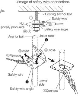
· When the existing anchor bolt that has been installed is used for connecting the safety wire, the use of 2 spacer nuts is helpful.
