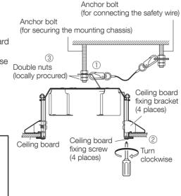
③ Use double nuts (locally procured) to secure the mounting chassis.
