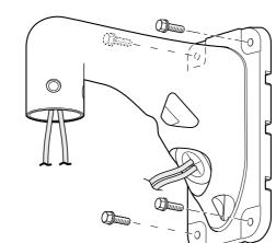
Apply a waterproofing to the holes for fixing this product on the wall.
