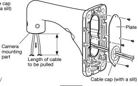
Mount this product on the wall with fixing screws (4pcs.) (M10: locally procured). Minimum pull-out strength: 823 N {185 lbf}/ per 1 pc.
