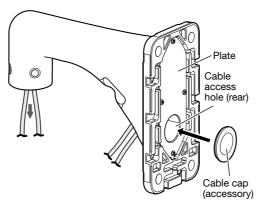
Seal the slit of the cable cap for the prevention of
