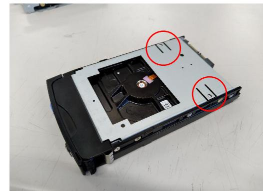
C and D places, fix with 2washers (③) and 2 screws (②)
