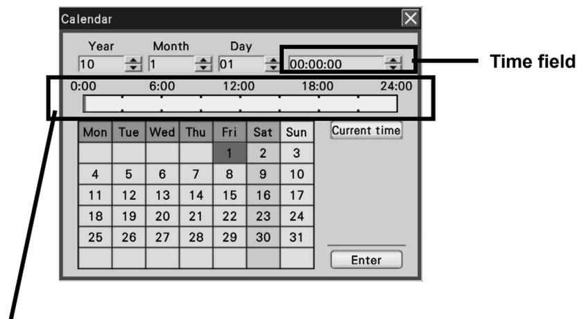
**Time input bar:** Click the mouse on the time input bar to input desired time related with clicked point by 15 minutes into the time field.
