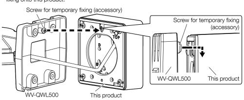
2 Fix WV-QWL500 on this product with four hexagon screws (M4: accessory) using a 3 mm hex wrench (locally procured).
