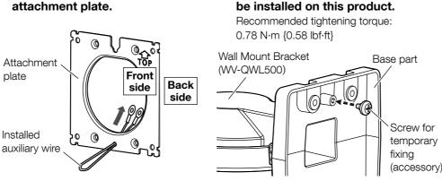
[3] If necessary, install the attachment plate provided with the camera to WV-QWL500 by following the instructions described in the Operating Instructions of WV-QWL500.
