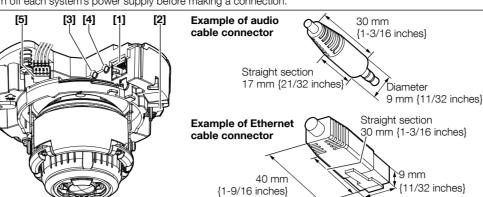
[1] Connect an Ethernet cable to the RJ45 network terminal
