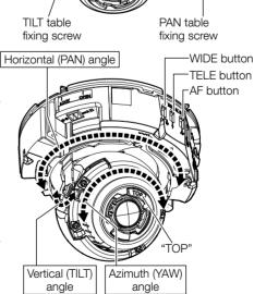
[4] Disconnect the MONITOR **OUT** conversion plug (accessory). Attach the enclosure and secure it by using a bit (accessory) to tighten the enclosure fixing screws (2 places).
