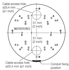
pattern from the following table and make holes. 85 mm {3-11/32 inches} **A** 85 mm {3-11/32 inches} (85.7 mm {3-3/8 inches}) (85.7 mm {3-3/8 inches}) **B** 138 mm {5-7/16 inches} 138 mm {5-7/16 inches} 46 mm {1-13/16 inches} **C** 83.5 mm {3-9/32 inches} **D** 63 mm {2-15/32 inches} 63 mm {2-15/32 inches} **E** Do not use Position E. **F** 70 mm {2-3/4 inches} 108.5 mm {4-9/32 inches}
