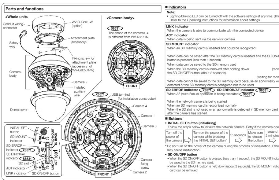
Lighting/blinking LED can be turned off with the software settings at any time. (The initial state is lighting or blinking.) Refer to the Operating instructions for information about settings.
