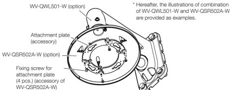
Fixing screw for attachment plate (4 pcs.)
