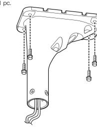
Apply a waterproofing to the holes for fixing this product on the ceiling and the cable inlet.
