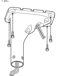
Apply a waterproofing to the holes for fixing this product on the ceiling.
