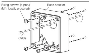
is an example when installing on a wall using the combination of the fixing screw holes that is 83.5 mm  $\{3-9/32 \text{ inches}\} \times$ 46 mm {1-13/16 inches}.
