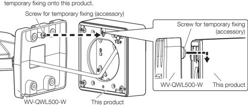
2 Fix WV-QWL500-W on this product with four hexagon screws (M4: accessory) using a 3 mm hex wrench (locally procured).
