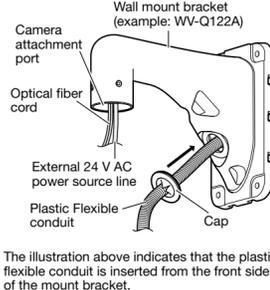
The illustration above indicates that the plastic flexible conduit is inserted from the front side of the mount bracket.
