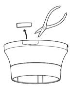
Attach the decorative cover by following step 10 of the "Wire through a hole in the ceiling" section (187 pages 22-23). Wire through the wiring hole of the decorative cover.
