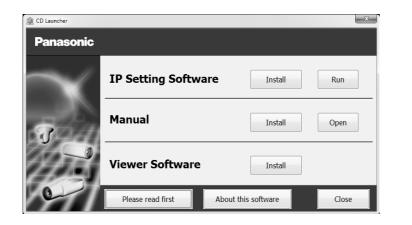
Click the [Run] button next to [IP Setting Software] "Panasonic IP Setting Software" page will be displayed. Click the [Network Settings] button after selecting the MAC address/IP address of the camera to be configured.
