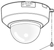
Dome cover fixing screw (M3, step screw)
