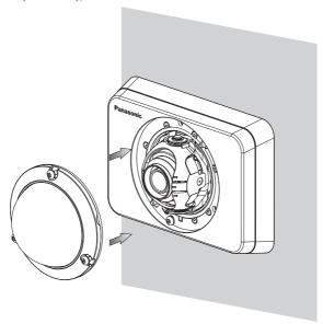
2 Remove the cover film completely.
