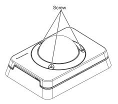
Remove the dome cover, dome cover ring and mount bracket.
