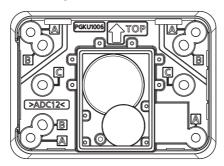
Mounting screw hole A: For standard mounting position on the wall Mounting screw hole B: For installing with a two-gang junction box Mounting screw hole C: For installing with a one-gang junction box
