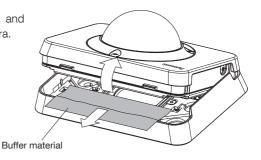
Loosen the 3 dome cover ring fixing screws (M3) using the tamperproof screw bit (accessory).
