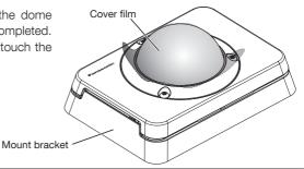
1 Separate the mount bracket and camera, and remove the buffer material out of the camera.
