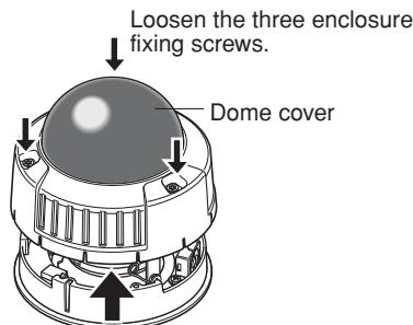
2. Detach the dome cover from the enclosure by removing the three dome cover fixing screws. (At this moment, the dome cover and the main body is still fixed with the dome wire. Remove the fixing screw of the dome wire.)
