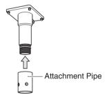
(2) Fix the attachment pipe to the bracket.
