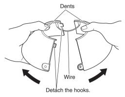
(2) Locate the front and rear sunshields to the position that covers the housing base.
