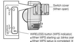
• When WPS starting up: blinks orange (for about 2 minutes) When WPS setup is completed: lit green
