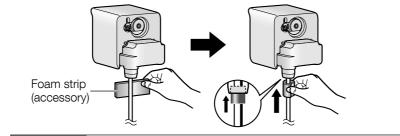
Adequate waterproof treatment is required for the cables when installing the camera outdoors. Failure to observe this may cause water leakage resulting in malfunction.
