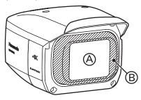
Meanwhile, residue of the coating gathers and remains around the surrounding area of Lens cover (Area-B) due to its construction method, but it does NOT affect the image quality too.
