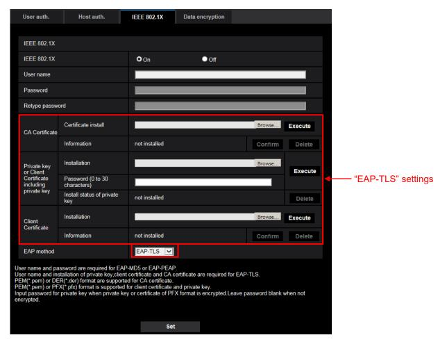
This function can be used to configure a secure network environment using the authentication LAN switch. Contact your network administrator for how to configure the authentication LAN switch and each setting.
