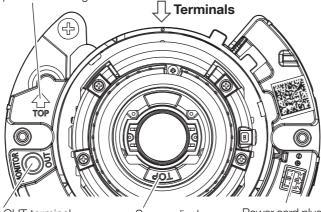
MONITOR OUT terminal (factory shipment: NTSC monitor) Screen display top (TOP)
