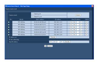
7 To change the IP address of the camera, enter a new IP address to the "New IP address" field and click the [Execute] button.
