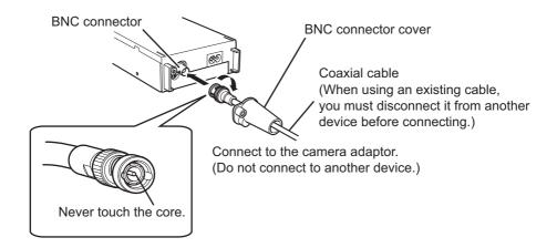
**6.** Secure the BNC connector cover with the included screw to the center adaptor. (Recommended torque 0.4-0.8 N·m {4.1-8.2 kgf·cm})
