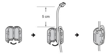
2. Connect a LAN cable (Cat-5e or higher) that is wrapped around a ferrite core to the camera adaptor and network camera.
