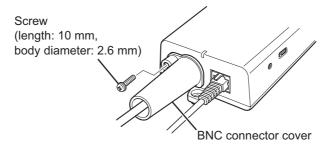
**5.** First pass the coaxial cable through the included BNC connector cover, then connect the coaxial cable to the BNC connector of the center adaptor.
