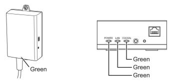
10. Press the center adaptor's SPEED button for about 1 second.
