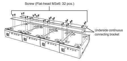
2. Secure the BY-HCA10CE mounting brackets to both sides of the connected center adaptors with the screws included with the BY-HCA10CE. (Recommended torque 0.4-1.0 N·m {4.1-10.2 kgf·cm})
