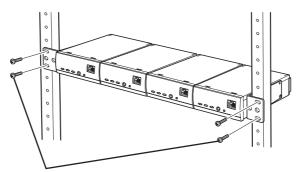
Rack mounting screw (customer-provided, nominal diameter 5 mm tapping)
