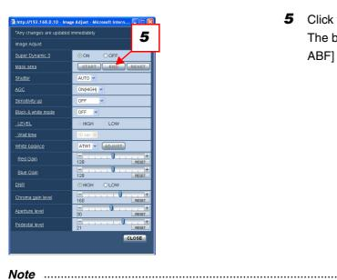
5 Click the [END] button after setting the mask areas. The borders on the image displayed on the [Image/ ABF] tab will disappear.
