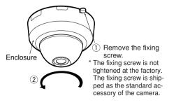
2. Detach the dome cover and the inner dome from the camera.
