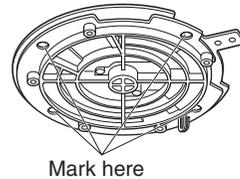
4. Affix the camera mounting base onto the ceiling.
