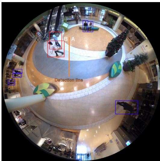
Intruder: An alarm is generated when a moving object enters the set area.
