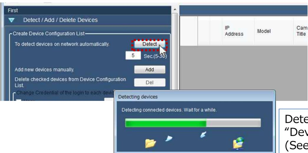
Detected devices shown up to "Device Configuration List" field.
