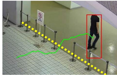
Figure 11: Cross Line Detection. Pre-defined detection line is shown in yellow for explanation.
