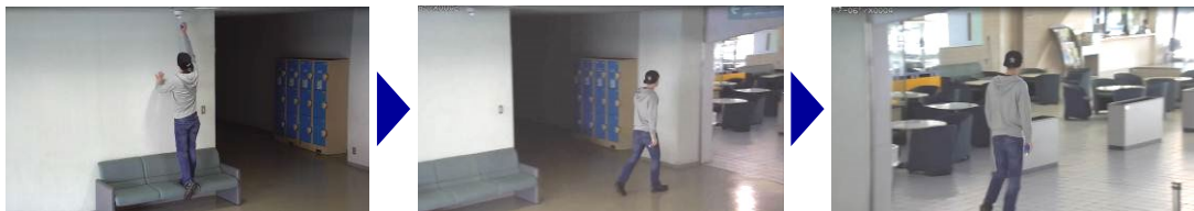
Figure 12: Advanced Auto Tracking and Scene Change Detection (i-VMD). In this example, when a camera was tampered, another PTZ camera started tracking by i-PRO inter-camera notification protocol from the tampered camera.
