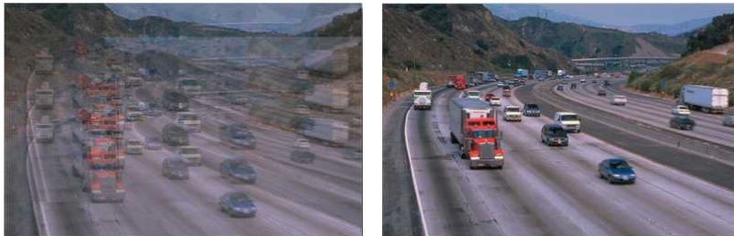
Figure 16: Free-way. At left, the image is blurred by vibration from the road. At right, Auto Image Stabilizer is on and eliminates the vibration effects.
