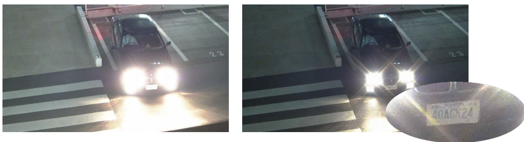
Figure 11: Vehicle front. At left, HLC is off. At left, High Light Compensation (HLC) suppresses excessive light and vehicle plate can be seen.
