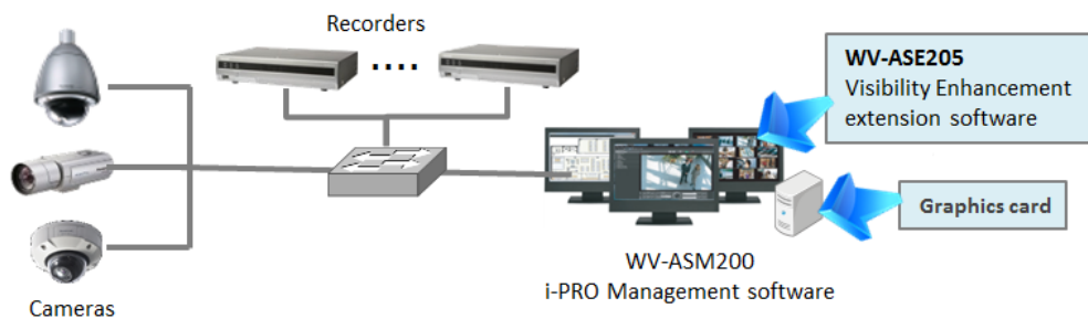
Figure 3: System configuration example of i-PRO Visibility Enhancement Software.
