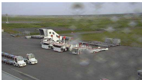
Figure 17: Airport on a rainy day. The left half of the dome cover is coated with Rain-Wash coating and the image is clear. For comparison, the right half is not coated.
