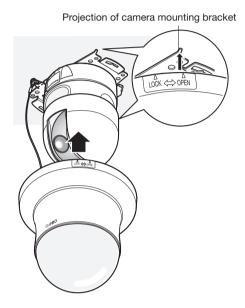
3 Turn this bracket clockwise until the projection of the camera mounting bracket aligns with "LOCK" of this bracket.
