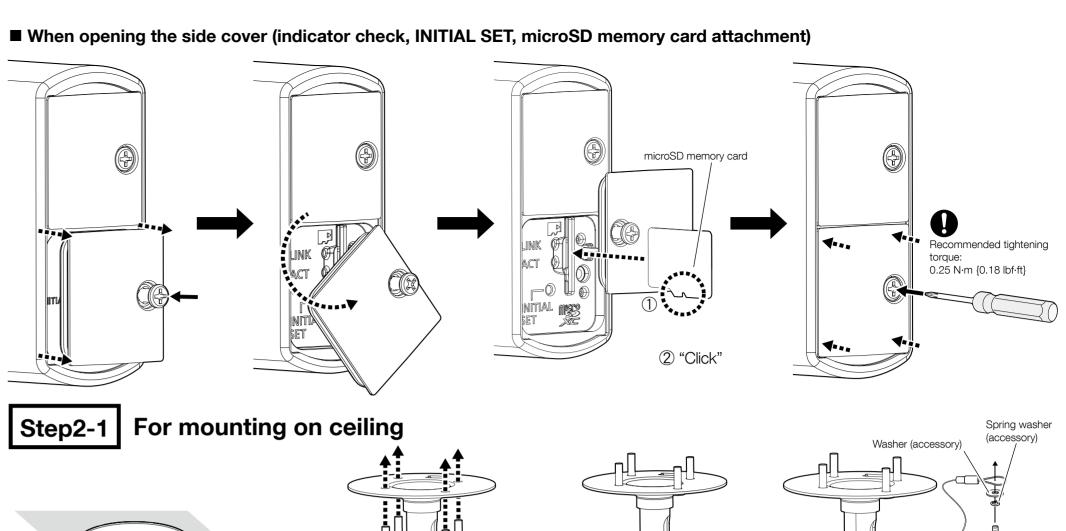
M6 (4 pcs.) (locally procured) Minimum pull-out strength: 562 N {126.34 lbf} (per 1 pc.) Fixing screw M4 (locally procured) Minimum pull-out
