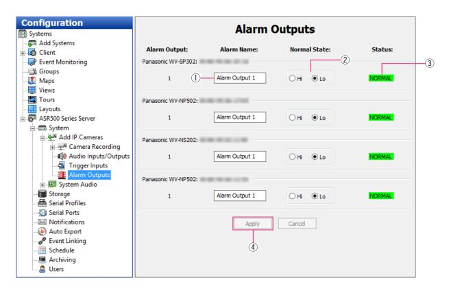
The "Alarm Outputs" page allows you to assign a name and configuration to the alarm outputs on hybrid systems and certain IP cameras.
