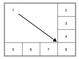
When no audio is assigned to any of the camera channels from which images are currently being displayed on a multiscreen, audio being input to audio input connector 1 (AUDIO IN 1) will be heard.
