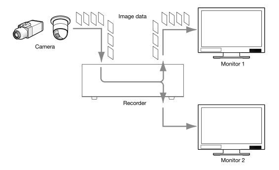
It is possible to display live images on a 1-screen or on a multiscreen. It is also possible to display live images from multiple cameras sequentially by switching the camera channels in order (sequence display). The audio will be output when images from the camera channel to which the audio is assigned are displayed on
