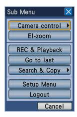
The "Sub Menu" window is the same window that can be displayed when operating the buttons on the front panel.
