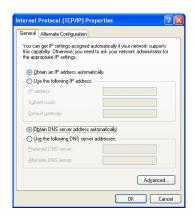
Depending on the network configuration, it is necessary to configure the default gateway. Refer to a system administrator for further information about the settings.
