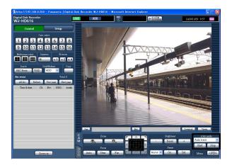
**Auto track:** The camera will automatically track an object moving on the screen.
