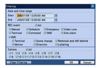
**Date and time range:** Designate the recording start time and date and the end time and date of recorded images to be searched for by rotating the jog dial (inside).
