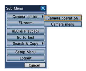
→ The "Camera menu" menu will be displayed and the camera setup menu will be displayed on the monitor.
