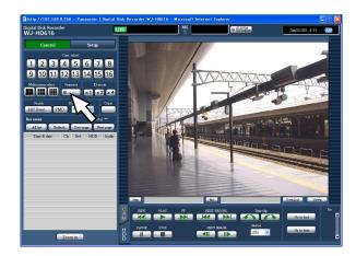
→ Live images from multiple cameras will be displayed sequentially according to the settings configured in advance. The indicator on the [Sequence] button will light green and the "SEQ" indication will be displayed on the status bar.
