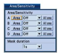
Up to 4 detection areas (A - D) can be set. It is also possible to set the whole displayed area as the detection area by pressing the [SET] button after moving the cursor onto the [Whole area] button.
