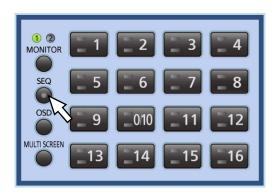
→ The sequence display will be performed according to the configured settings.
