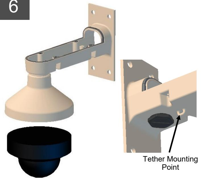
Attach the camera to the pendant shroud and complete all wiring connections inside the mount.
