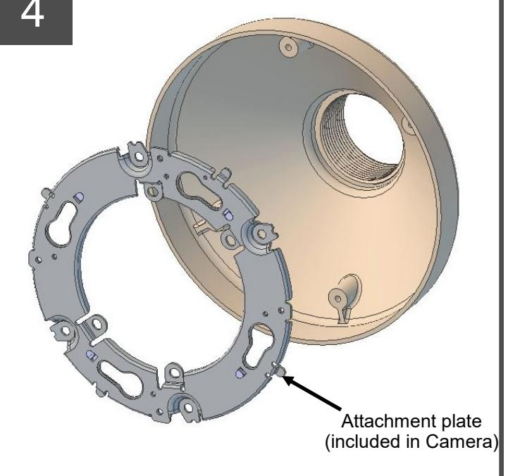
Install attachment plate into pendant shroud using the provided (8-32) screws.
