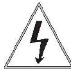
The lightning flash with an arrowhead symbol, within an equilateral triangle, is intended to alert the user to the presence of non-insulated "dangerous voltage" within the product's enclosure that may be of sufficient magnitude to constitute a risk of electric shock to persons.
