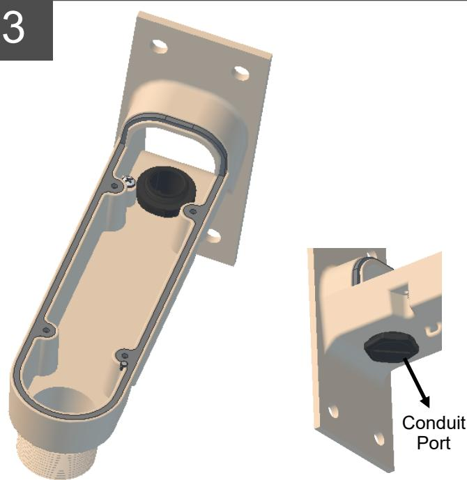
Pull the appropriate camera cabling into the wall mount.
