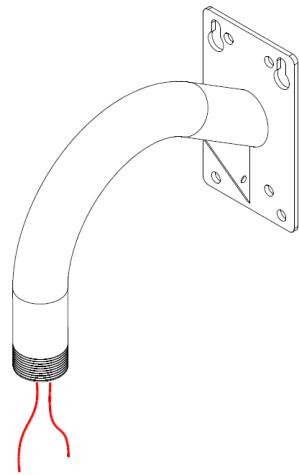
Securely mount bracket to wall using appropriate fasteners. Pull wiring through bracket.
