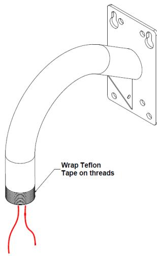
Wrap Teflon tape around the pipe threads to ensure a tight seal.
