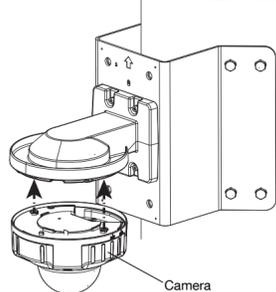
**C Install the camera by using this product with Wall Mount Bracket (WV-QWL500) and Adapter Box (WV-QJB500).**
