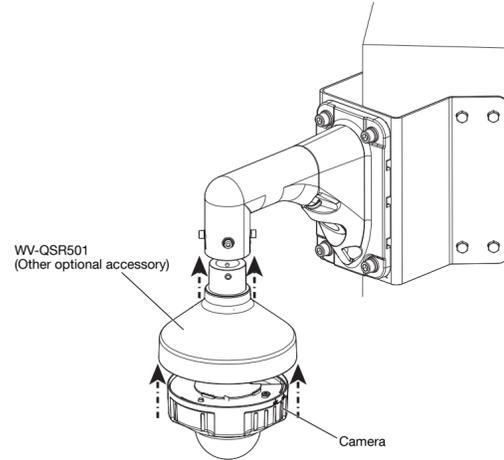
**B Install the camera by using this product and Wall Mount Bracket (WV-QWL500).**
