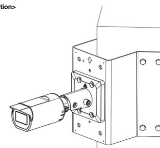
**E Install the camera by using this product and Adapter Box (WV-QJB500).**
