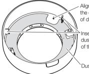
Align the microphone hole of the enclosure with the notch of dustproof sheet.
