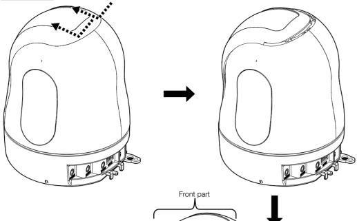
• The front part is secured with hooks. Push the top of the front part downward at an angle from the top of the camera, remove the hooks in order from the top, and remove forward.
