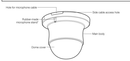
\* If a tiepin type microphone is used, mount the microphone on the rubber-made microphone stand. Unless the microphone is used, cut the rubber with a nipper or conduct another treatment.
