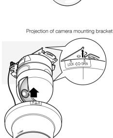
② Attach the inner cover. ③ Turn this product clockwise until the projection of the camera mounting bracket aligns with "LOCK" of this product.
