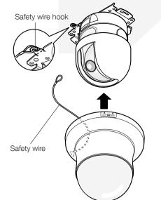
② Mount this product on the camera with aligning the projection of the camera mounting bracket (2 places) with "OPEN" of this product (2 places).
