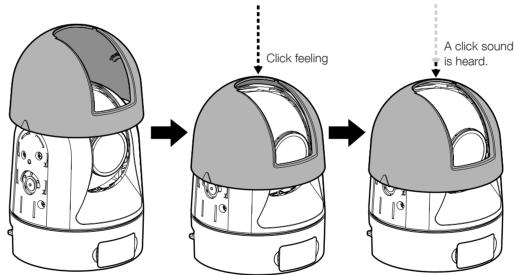
■ When removing the inner cover Release the claws on the inner surface on both the left and right sides one by one and then remove the inner cover.
