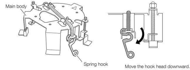
**■ Fix the attachment plate (camera accessory) to the ceiling mount bracket.**
