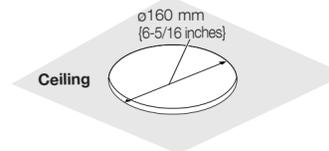
**Step2 Fix the ceiling mount bracket onto the ceiling board.**
