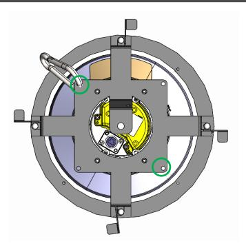
Attach Camera Safety Tether to the opposite corners which are not being used for safety tethers at Step-4A
