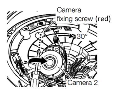
Use the driver bit (supplied with the camera) to loosen the screws and remove the enclosure from the camera main body.
