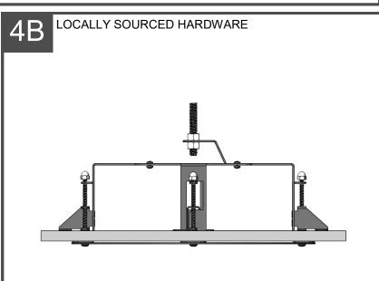
Install (1) Anchor bolt into ceiling and measure distance appropriate for mount. Place (1) Hex Head 3/8"-16 nut above mounting hole in mount and (1) below mount.
